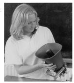
Carol calculates that she can safely turn the power supply up to 10 volts without destroying the voice coil, but at 10 volts the speaker hums widly. She turns the voltage down to 6 volts which gives a steady 50 cycle hum.
